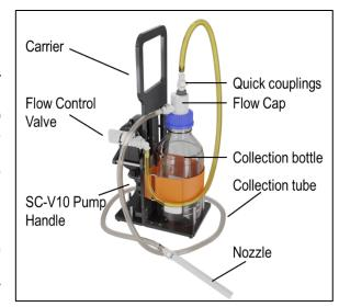
Components are designed for ease of assembly, operation, and disassembly by users wearing heavy gloves in the field. Following sample collection, the device's wetted tubing and collection vessel can be separated, the vessel capped, and all pieces bagged, to prevent sample loss or cross-contamination.
